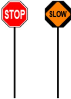
Illumination shall be provided for Traffic Control Persons required to be working on or adjacent to City ROW during hours of darkness. Always use the appropriate Traffic Control Person Ahead sign (TC-21) and all other required signage/delineation. Traffic Control Persons shall stop traffic from the side of the traffic lane and shall never turn their back to traffic. Traffic Control Persons shall never leave their post until relieved by another Traffic Control Person in full safety gear.
