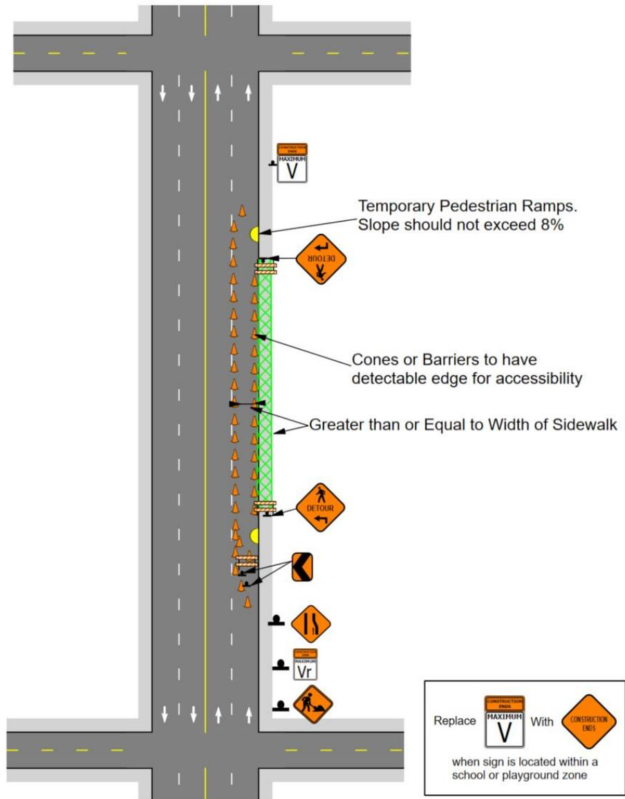
Drawing 31: Sidewalk Intersection Closure with Detour
