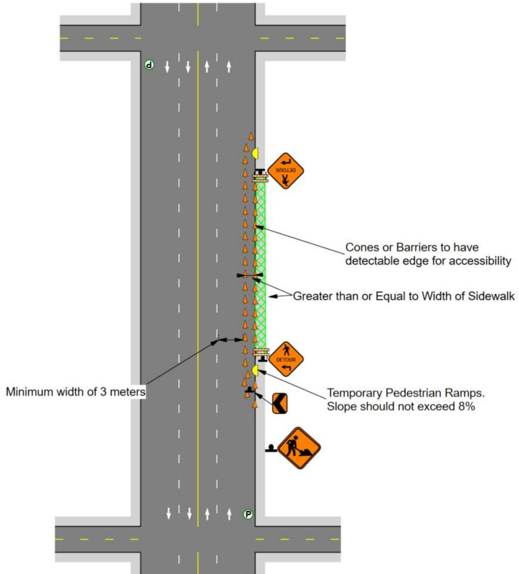
Drawing 30: Sidewalk Closure with Driving Lane Detour
